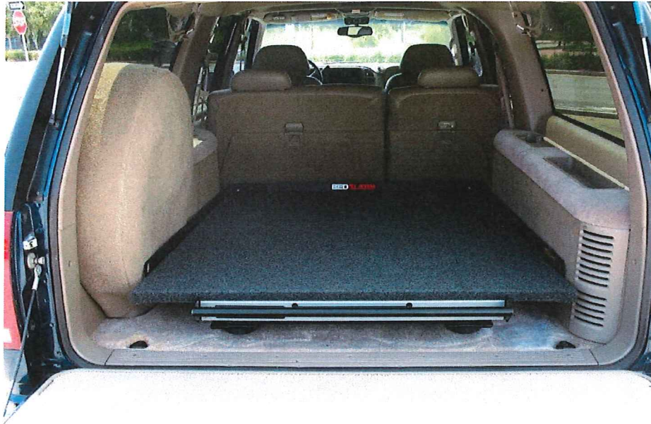
Photos of Sliding Racks Installed in SUV
